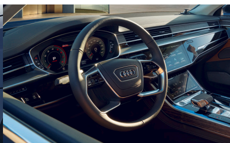
Twin-spoke leather multifunction steering wheel with shift paddles, electric tilt and axial adjustment
